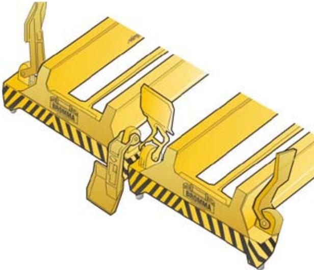
The spreader is equipped with eight powerful flipper arms, two middle flippers and two side flippers on each spreader.
