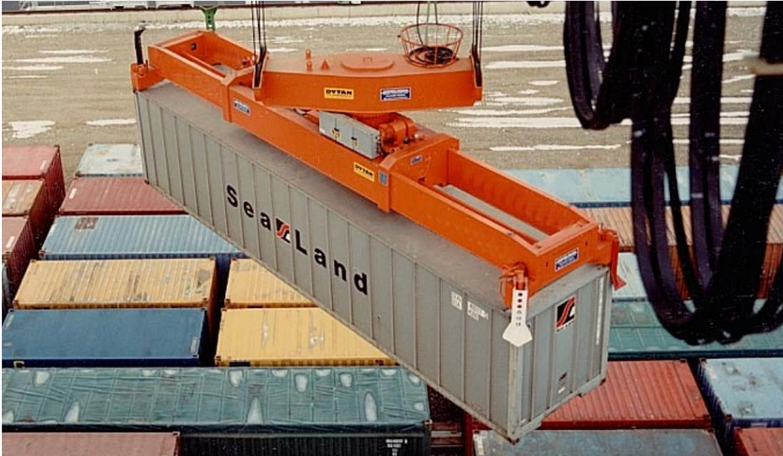
Bromma's EH7 rotating telescopic spreader with gravity point adjustment is ideal for the handling of off-centre container loads. The unit is often used for the purpose of rotating a container through 180 degrees to ensure that the container is placed in the correct way on a trailer or rail car. The EH7 is used in conjunction with the Bromma EH9 rotator.
